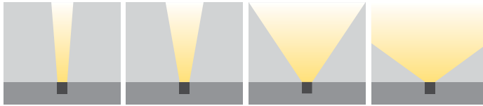
XN: Extra Narrow Angle N: Narrow Angle W: Wide angle XW: Without lens
