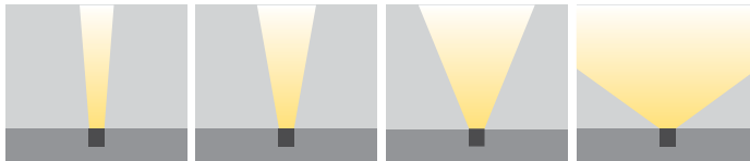
XN: Extra Narrow Angle N: Narrow Angle M: Medium Angle XW: Without lens
