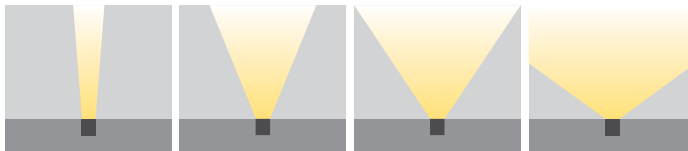
XN: Extra Narrow Angle M: Medium Angle W: Wide angle XW: Without lens
