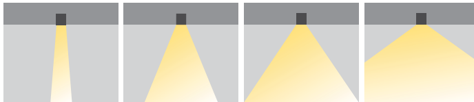
XN: Extra Narrow Angle M: Medium Angle W: Wide Angle XW: Without lens
