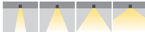
N: Narrow Angle M: Medium Angle W: Wide Angle XW: Without lens
