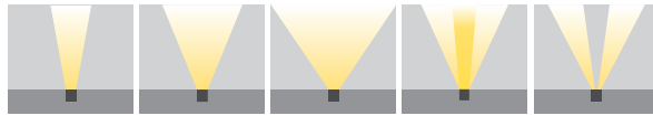
N: Narrow Angle M: Medium Angle W: Wide Angle E: Elliptical Angle OAS: Double Asymmetrical Angle
