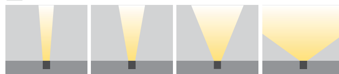
XN: Extra Narrow Angle N: Narrow Angle M: Medium Angle XW: Without lens
