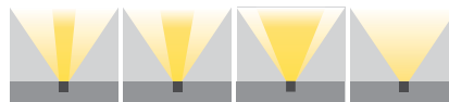
XN: Extra Narrow Elliptical Angle N: Narrow Elliptical Angle M: Medium Elliptical Angle W: Wide Angle
